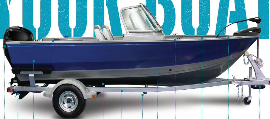
motor prop bilge live-wells axle bunks trailer rollers hull dock-lines bait bucket anchor prop
